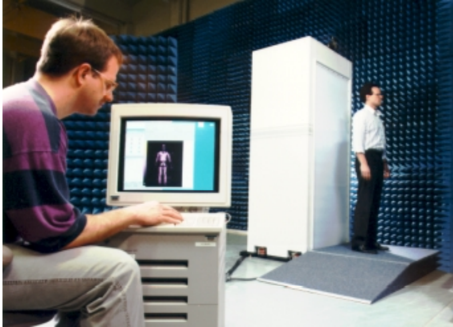
Figure 2 Prototype wideband millimeter-wave imaging system.
