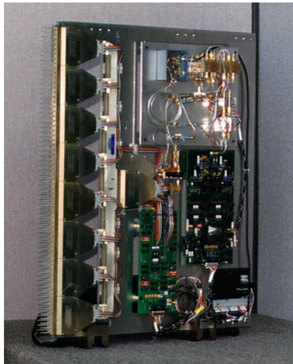
Figure 3 128 element, 27 - 33 GHz millimeter-wave linear array.
