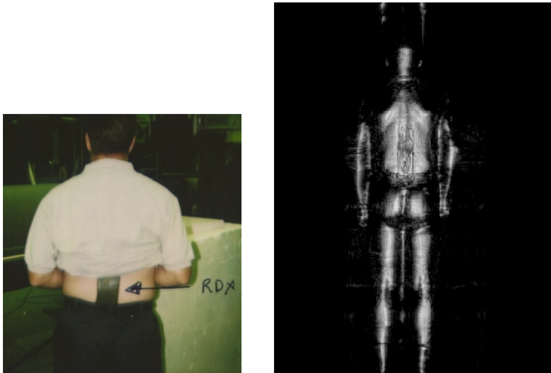
Figure 9 Wideband (27 - 33 GHz) images of a man carrying a concealed block of RDX ‘plastic’ explosive near the center of his back. (a) Optical picture (b) Millimeter-wave image.
