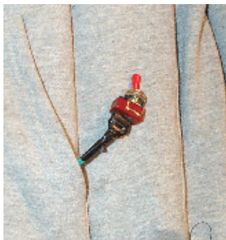
Typical Initiation Switch, Concealed in Pocket of Vest
