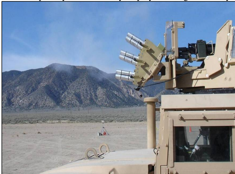
Figure 1: VENOM mounted on gun turret of an up-armored HMMWV.
