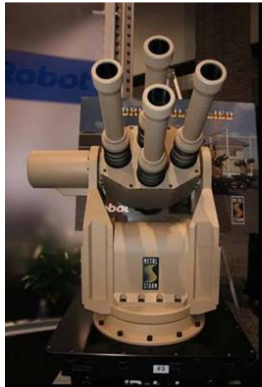
Figure 4: One prototype for the Mission Payload Module will be based on this multi-barrelled grenade launcher.
