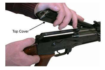
Figure 21. Installing the Top Cover.
