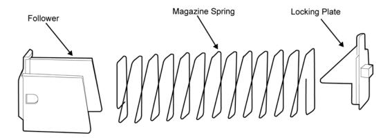
Figure 26. Follower, Magazine Spring, and Locking Plate Removed.
