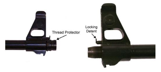
Figure 13. Thread Protector and Locking Detent.
