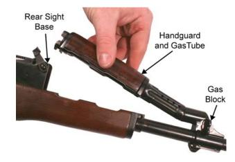
Figure 16. Inserting the Gas Tube.
