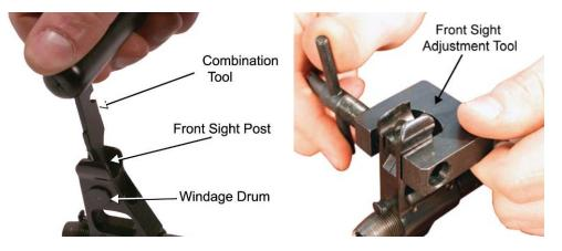
Figure 4. Setting the Front Sight Post and the Windage Drum.
