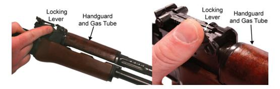
Figure 10. Pushing the Locking Lever to the Up Position.
