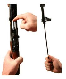
Figure 4. Running the Bore Brush though the Bore and out of the Muzzle.
