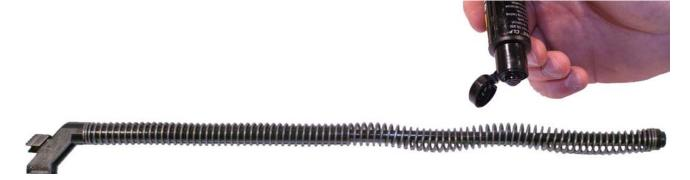
Figure 5. Lubricating the Recoil Spring and Guide Rod Assembly.
