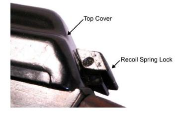
Figure 5. Two-Piece Recoil Spring Lock.
