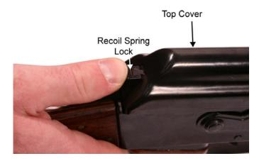
Figure 4. Pushing in the Recoil Spring Lock.
