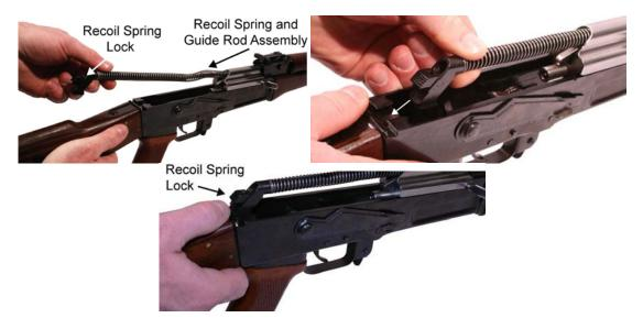
Figure 20. Installing the Recoil Spring and Guide Rod.
