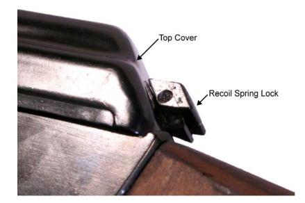
Figure 22. Two-Piece Recoil Spring Lock.
