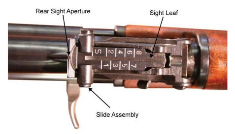
Figure 5. The Rear Sight with the Slide Assembly Set on the "S" Setting.
