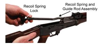
Figure 7. Lifting the Recoil Spring and Guide Rod Assembly Up and Out of the Receiver.
