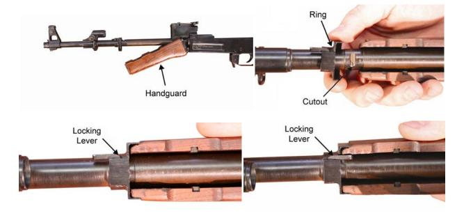
Figure 15. Installing the Handguard.
