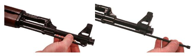
Figure 3. Removing the Cleaning Rod.
