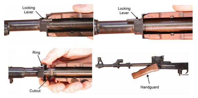
Figure 12. Removing the Handguard.
