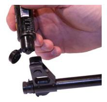
Figure 2. Lubricating the Front Sight Post.
