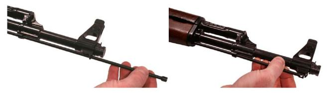
Figure 23. Installing the Cleaning Rod.
