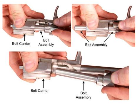
Figure 9. Removing the Bolt Assembly.
