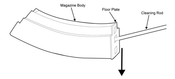
Figure 25. Pushing in the Locking Plate and Sliding the Floor Plate off of the Magazine.
