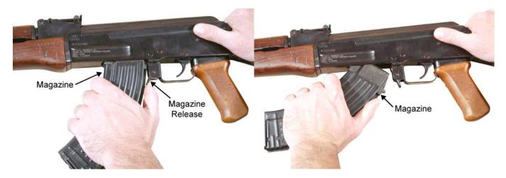
Figure 2. Removing the Magazine.
