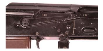
Figure 6. Selector Lever Placed on SAFE.
