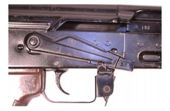
Figure 7. The Selector Lever Placed on SEMI.
