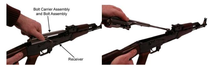
Figure 8. Removing the Bolt Carrier Assembly and Bolt Assembly.
