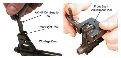
Figure 3. Using the Front Sight and the AK-47 Front Sight Adjustment Tool.
