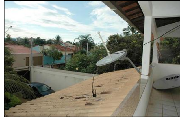
Homemade Brazilian SAT uplink used to pirate FLTSATCOM transponders
