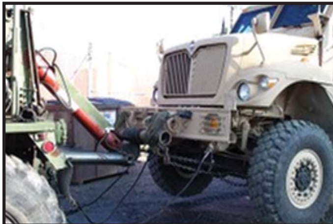
Figure A-32: HEMTT/MTVR wrecker front lift towing IMG MaxxPro
