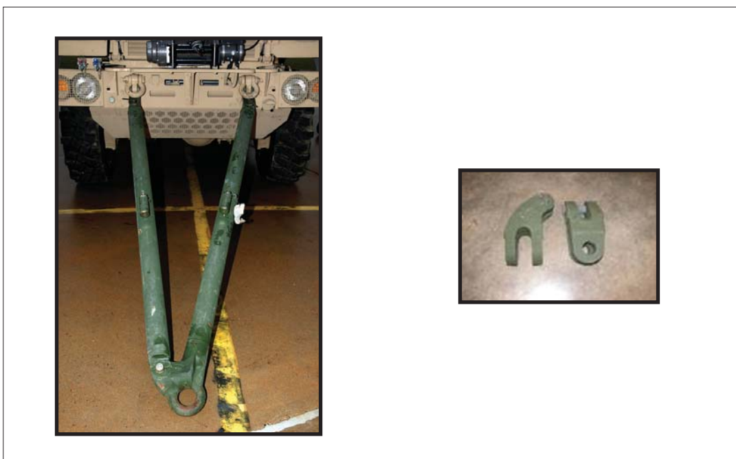
Figure A-12: U.S. Army heavy duty towbar (NSN 2540-01-267-2912) and adapter (NSN 2540-00-863-3153)
