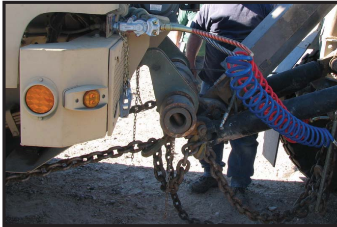
Figure A-15: HEMTT/MTVR wrecker front lift tow with HEMTT BII adapter F (NSN 2590-01-226-3351 [L] and NSN 2590-01-226-3350 [R])
