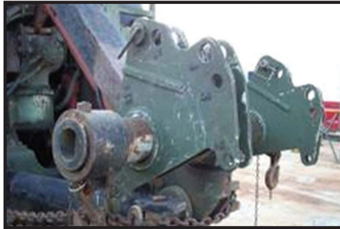
Figure A-34: HEMTT/MTVR wrecker with MUAs (NSN 5340-01-516-2058 [L] and NSN 5340-01-516-2059 [R])
