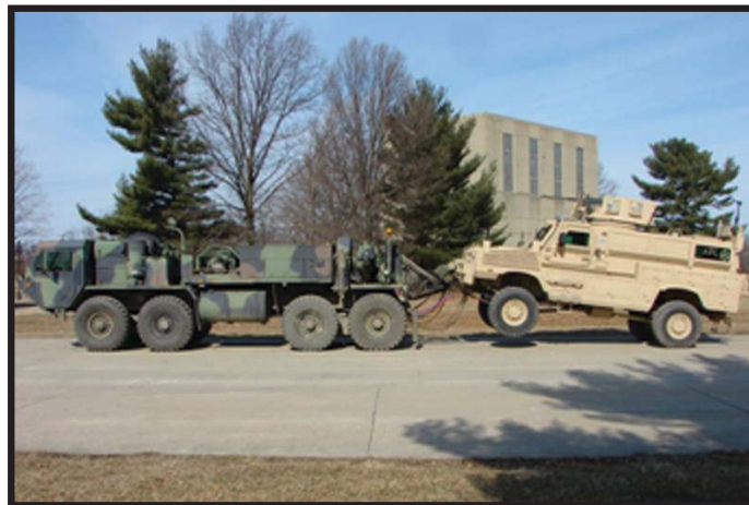
Figure A-42: HEMTT wrecker lift towing GDLS
