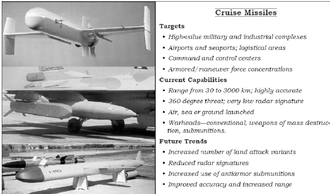
Figure B-5. Characteristics of cruise missiles
