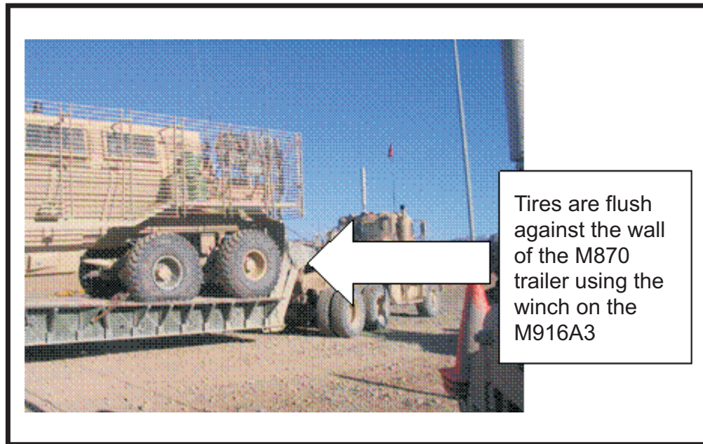
Figure 5-2. Using the winch on the M916A3 tractor, the maintenance crew brings the rear tires of the Buffalo up flush against the now-raised gooseneck of the M870 trailer.
