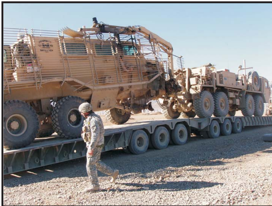
Figure 5-1. HEMTT wrecker lifts and tows disabled Buffalo onto M870 trailer.
