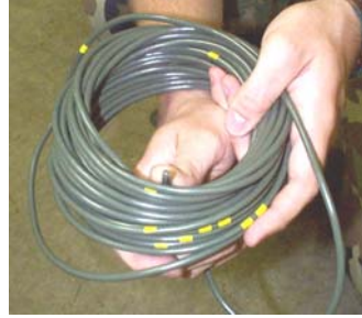
Figure 1.4. Roll of M700 Time Fuze
