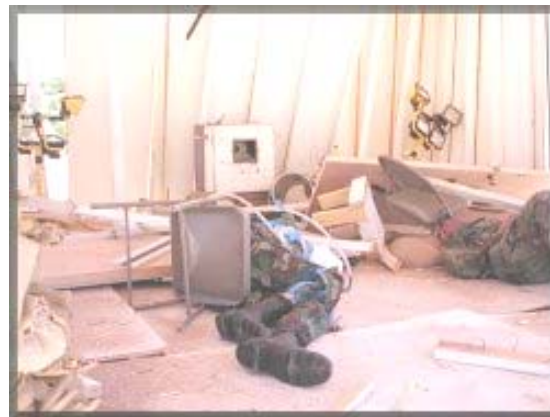
Figure A4.14. BAIT Post-test SEA Hut Post-test Anthropomorphic and Cadaver Setup Inside a SEA Hut
