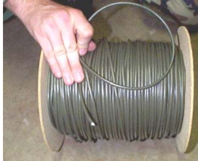
Figure 1.7. Typical Roll of Military Det Cord
