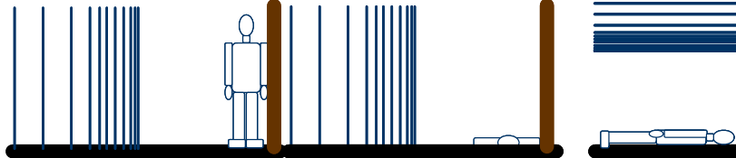
Figure 4.2. Thorax Near a Reflecting Surface Which is Perpendicular to Blast Winds, Subject Facing Any Direction
