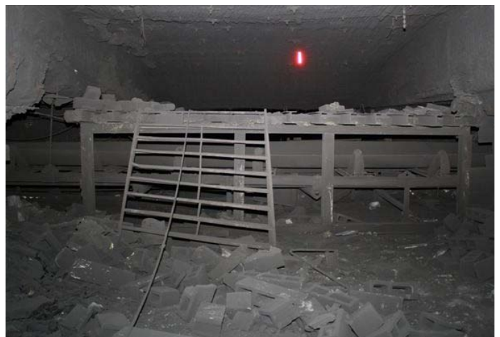
Above, the mantrip in which the Tailgate 22 crew was riding; below, the remains of a cinderblock wall gives an indication of the force of the explosion.
