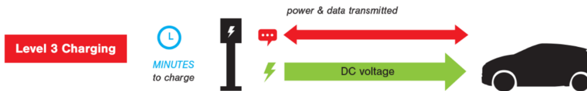
FIGURE 5—LEVEL 3 FAST CHARGING DIRECT CURRENT
