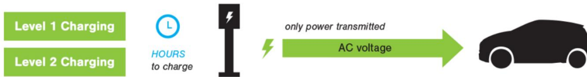
FIGURE 4—LEVELS 1 AND 2 SLOW CHARGING AC
