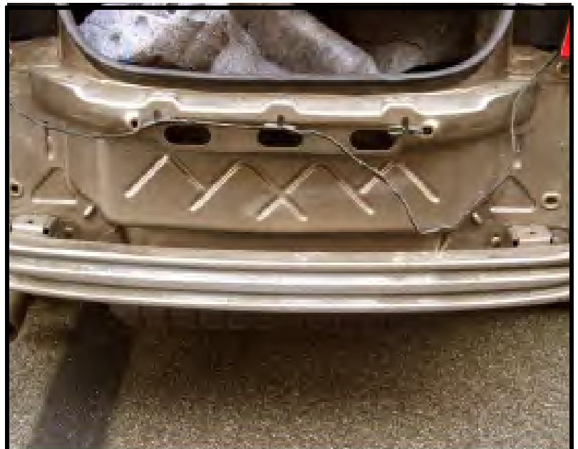
close-up of trunk structure and actual rear metal bumper
