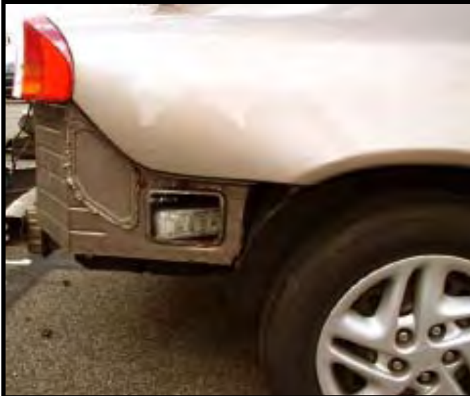
Right side of trunk with access panel removed
