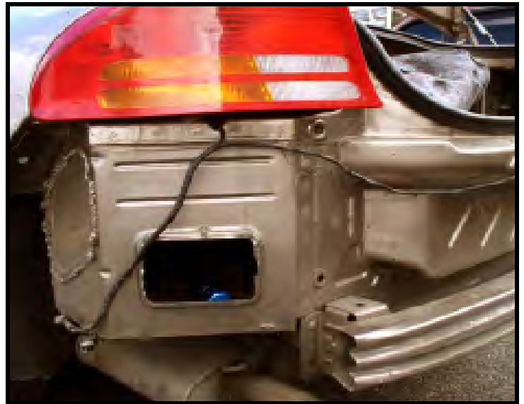
Left rear corner of trunk with access panel removed
