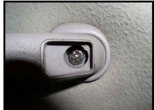
Close Up Of Screw with Burn Marks
