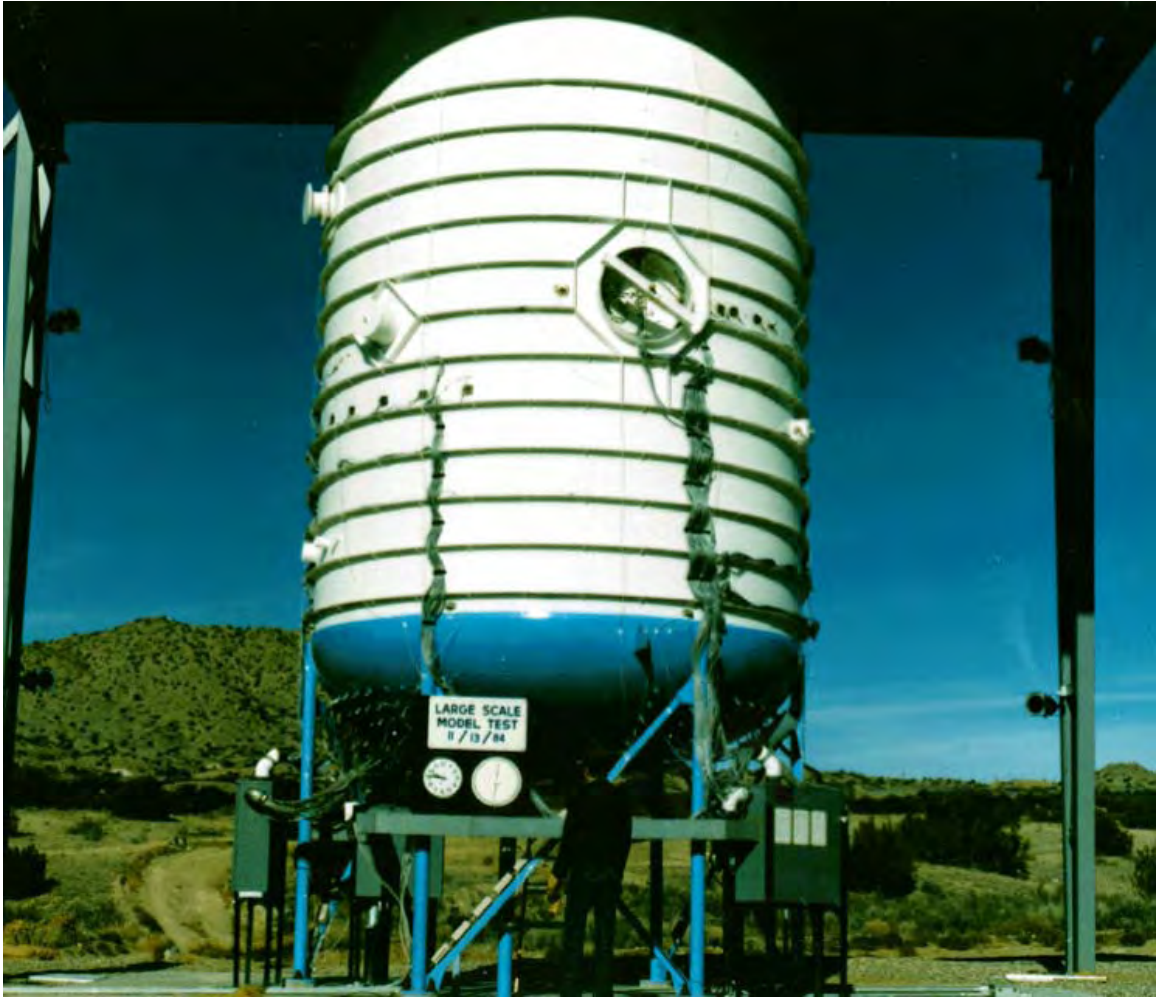
Figure 26 1:8-Scale Steel Containment Model
