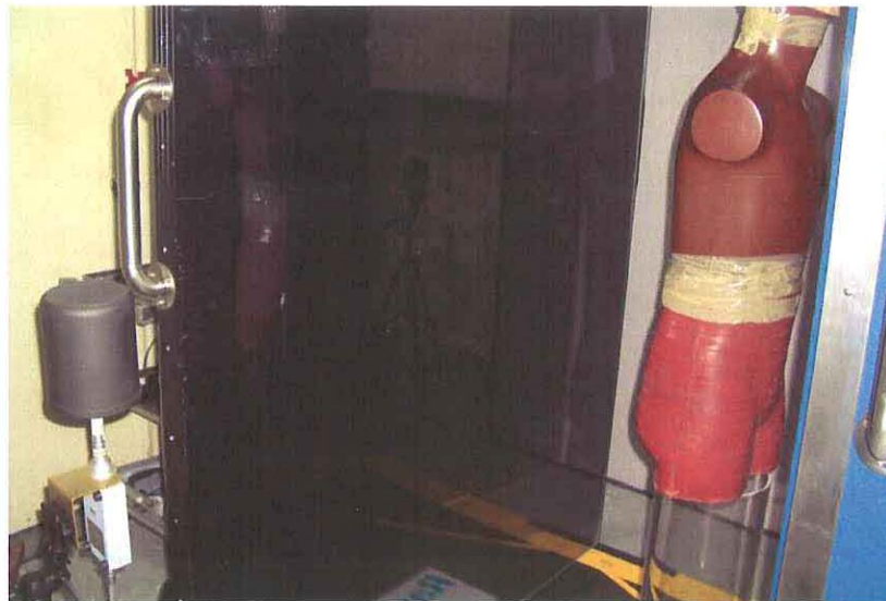
Figure 14. Measurement of scatter exposure, location (2). The exposure at this location was 0.11 \mu\text{R}/\text{scan} .
