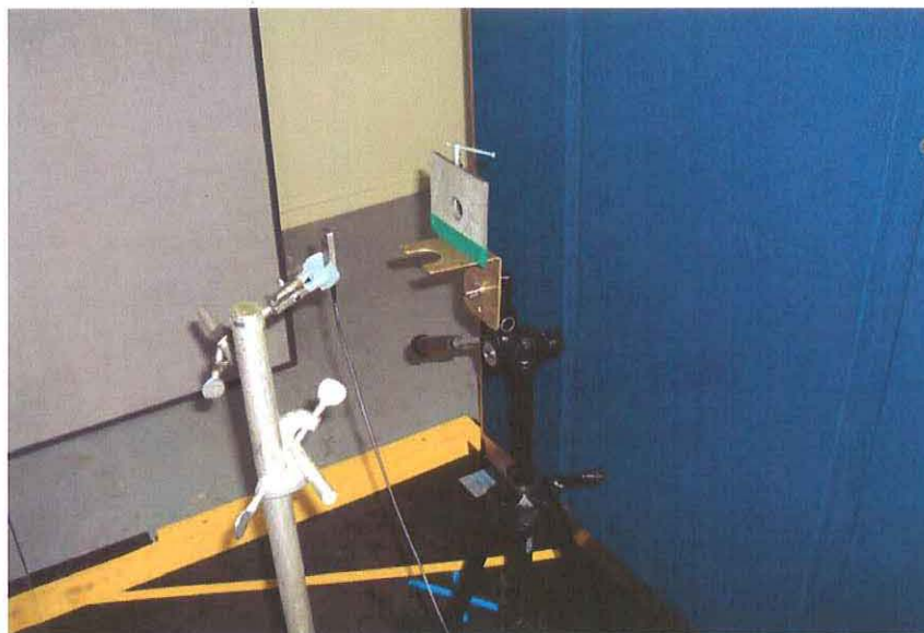
Figure 2. Setup for the HVL measurement. The aluminum attenuators were placed against the lead collimator.
