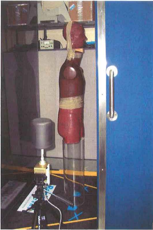
Figure 12. Measurement of scatter exposure, location (1). The exposure at this location was 0.20 \mu\text{R}/\text{scan} .
