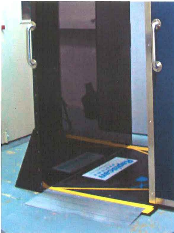
Figure 15. The back plate assembly showing the handle and the triangular aluminum plate mounted on the outside foot. The outside foot protrudes 29 cm behind the plate. The inside foot is covered by the aluminum ramp.
