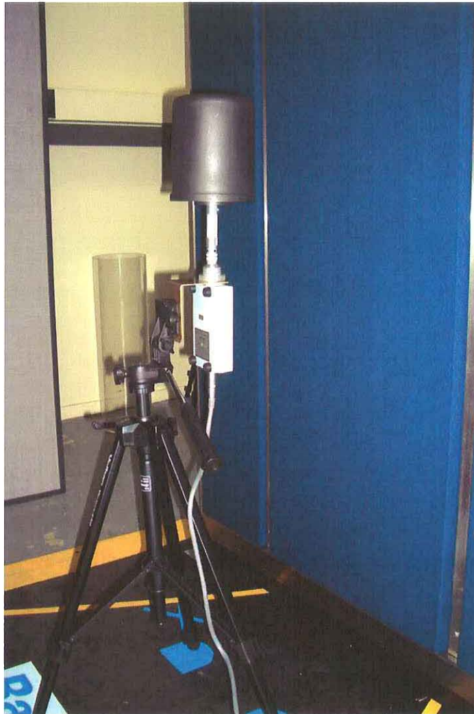
Figure 10. Measurement of the exposure using the 1800 cc ionization chamber.
