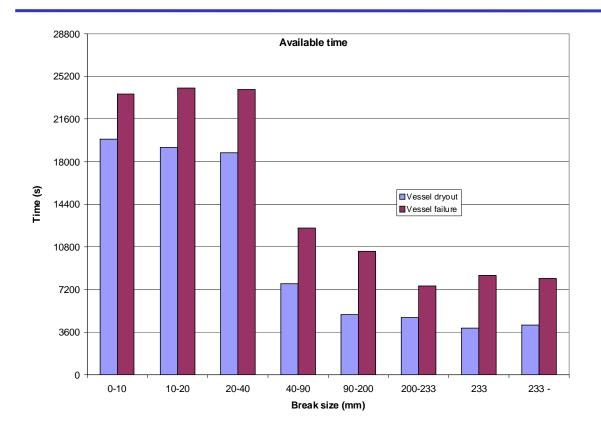
Available time for flooding the cavity from the signal T<sub>EXIT</sub>=1100 C
