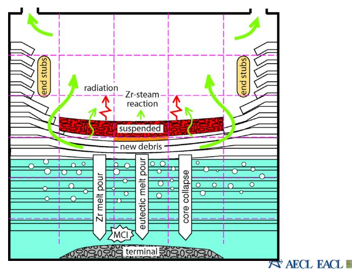
Consolidated terminal debris bed; beginning of molten corium formation near the top surface and the evolution of natural circulation in the reactor vault water
