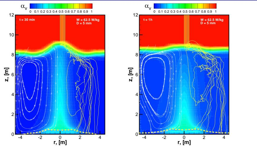
Flowfields and debris bed shapes (shown by yellow dashed line) at 30 min and 1 hour
