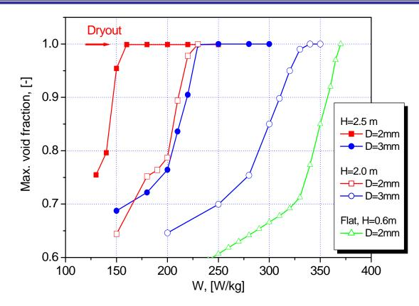
Maximum void fraction vs Specific heat release rate for different particle diameters and debris bed heights, as well as for a 0.6 m high flat layer (with the same total mass of debris)
