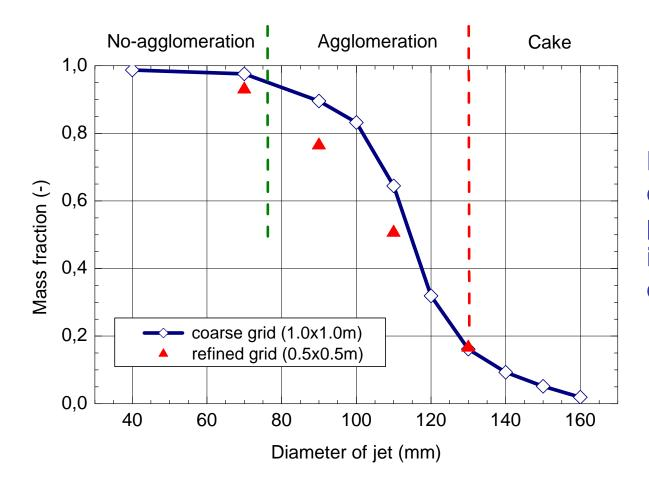
Rapid decrease of completely solid particle fraction with increase of the jet diameter
