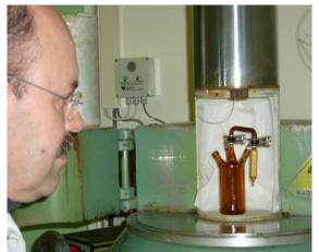
Photo of reaction vessel in  $\gamma$ -irradiation chamber
