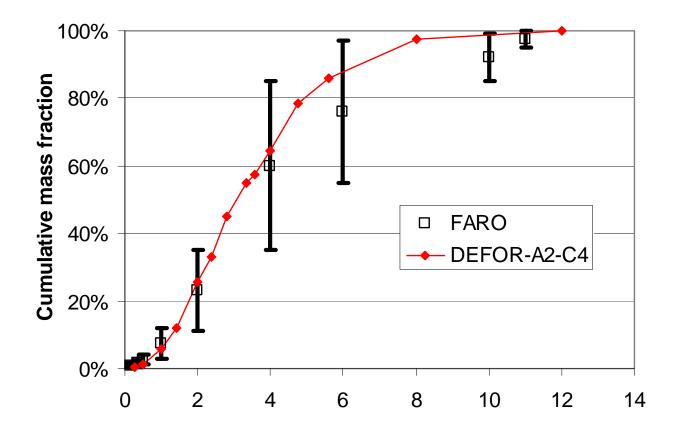
Particle size distribution in DEFOR agrees well with data obtained in the FCI experiments with real corium
