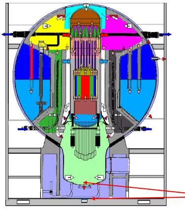
each coloured cell = one CV node of input deck
