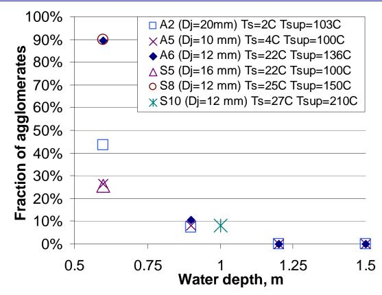
Fraction of agglomerated debris is lower in tests with low water subcooling and with bigger jet diameter
