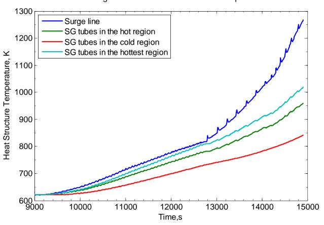
Surge line and SG heat structure temperature
