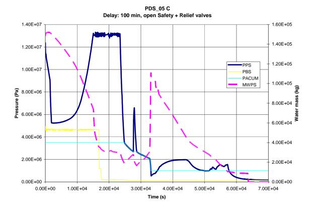
Primary system pressure (PPS) and water mass (MWPS) in the vessel in case of primary system depressurization at 100 min after the signal TEXIT = 550 C
