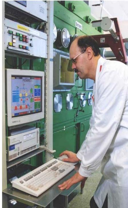
In the shielded cell of the Hot Lab... a computerized, remote-operating system has been installed
