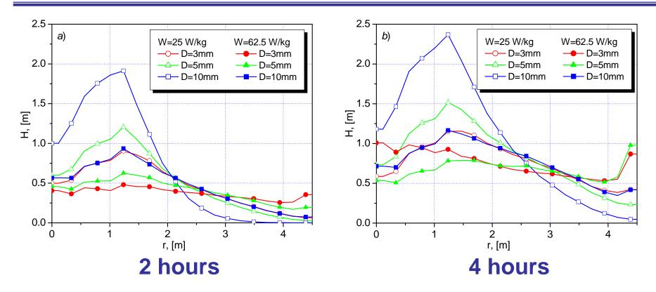
Natural convection flows promote flattening of debris bed, especially for fine particles
