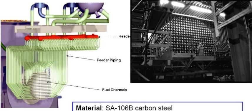
Material: SA-106B carbon steel Pipe Size: NPS 1.5 (DN 40) through NPS 3.5 (DN 90) Length: 20 feet (6.1 m) through 60 feet (18.3 m) Operating Pressure: nominally 9 to 11 MPa Operating Temperature: nominally 250 to 310°C
