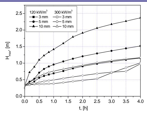
Stronger convective flows result in particle spreading over the pool bottom, especially for fine particles
