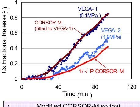
Modified CORSOR-M so that calculation at 0.1MPa might agree with the measurement
