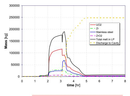
Melt mass in the LP and Melt ejection
