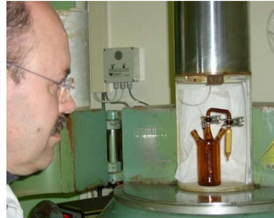
Photo of reaction vessel in  $\gamma$ -irradiation chamber and gamma-cell
