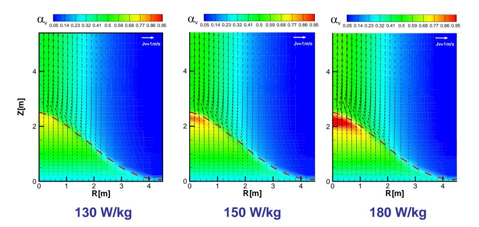
Void fraction distributions in the debris bed for different specific heat release rates
