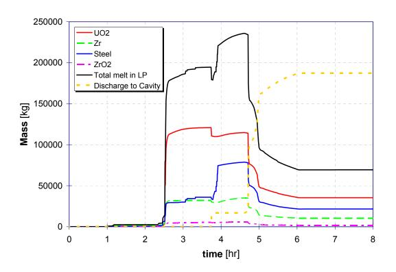
Melt mass in the LP and Melt ejection
