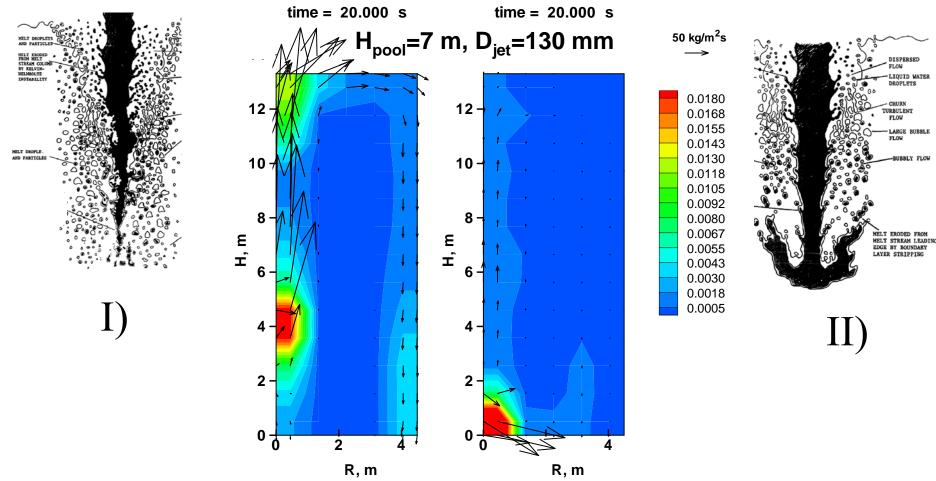
Completely different dynamics of particle motion and solidification:
