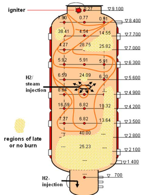
Fig. 5-4: Flame front propagation as isochrones:
