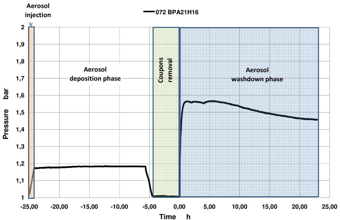
Fig. 5-7: Aerosol Wash-Down Test: Test phases
