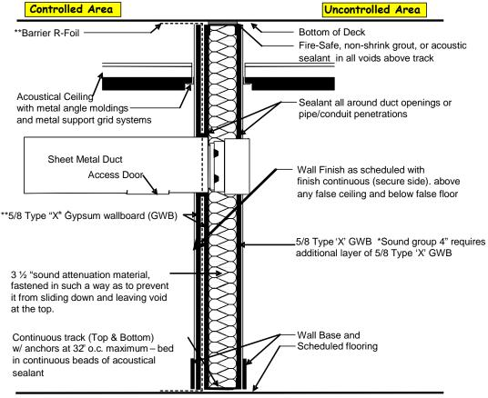
Conduit pipe penetrations should be sealed all around.
