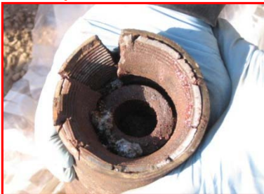
Example - Central burster charge visible
