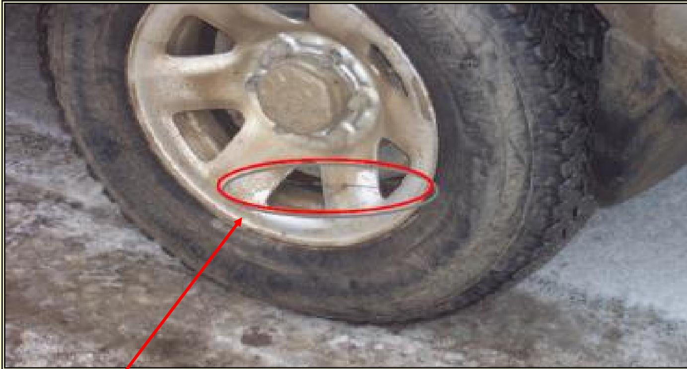
VICTIM OPERATED (INITIATED) BOOBY TRAP; IED DETONATES AS CAR MOVES; MOST LIKELY IMPROVISED GRENADE DEVICE OR PLASTIC EXPLOSIVE; NOTICE EXPOSED WIRE.
