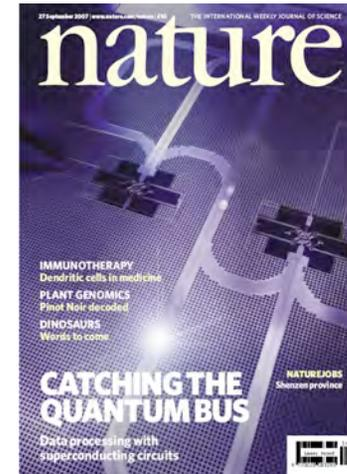
Cover and illustration show two SC qubits coupled by a serpentine waveguide resonant cavity.
