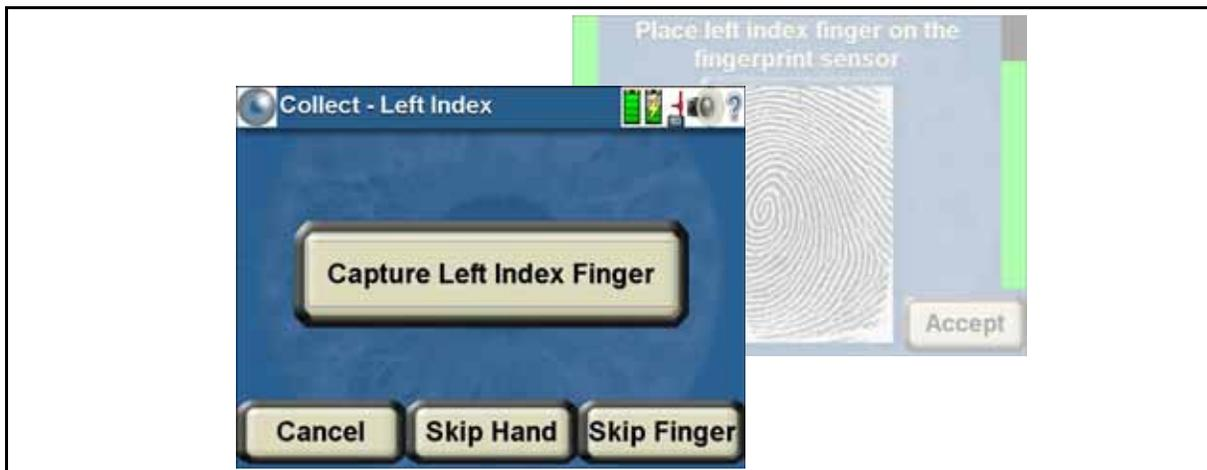
With the fingerprint capture screen active, have the subject put a fingerprint on the fingerprint sensor, located on top of the HIIDE. The preview window displays the fingerprint. To complete enrollment of that finger press the “**Accept**” button, or one of the shoulder triggers.
