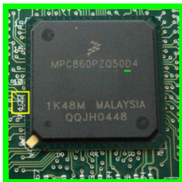
Figure 2. 2600XM: Compliant units use a microprocessor at U22 of the PCB whose part number has a “D” as the second-to-last character, such as XPC860PZP50D4.
