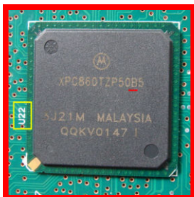
Figure 1. 2600XM: Certain counterfeit units use an incorrect microprocessor at U22, with a part number that has a “B” as the second-to-last character.
