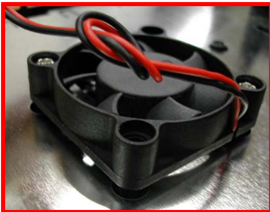
Figure 9. 1721: Non-compliant fan has no part number sticker
