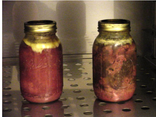
Mock-Up of Inoculated (Right) and Uninoculated (Left) Jars After Incubation
