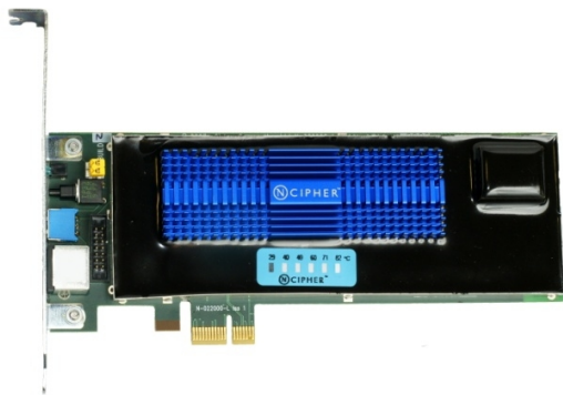
Figure: NCipher nShield F3 Hardware Security Module in the form of a PCI card
