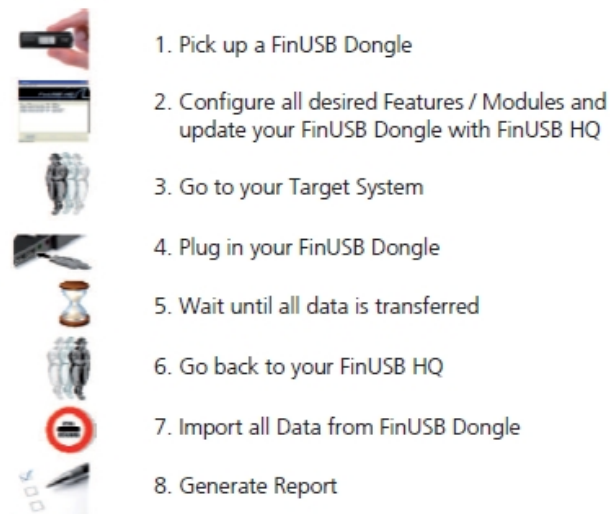
Figure 14: Steps for using FinUSB (source GammaGroup)
