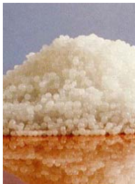
(U) Prilled Ammonium Nitrate
