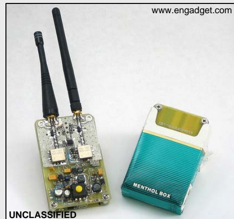
(U) Portable radio frequency jammer hidden in cigarette pack.
