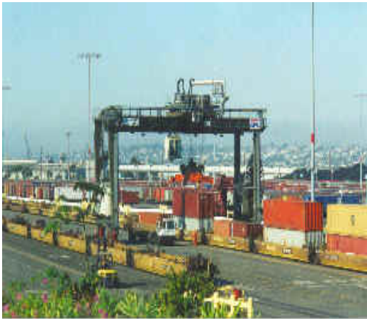
Figure 7 Intermodal Section of a Rail Yard with Crane and Loader
