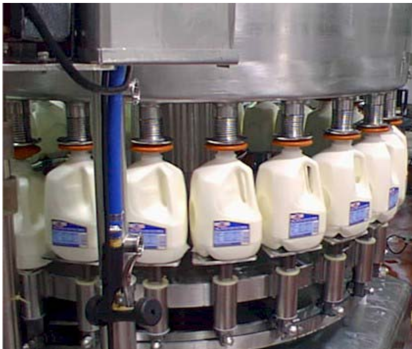
Figure 9 Machine for Filling Milk Jugs
