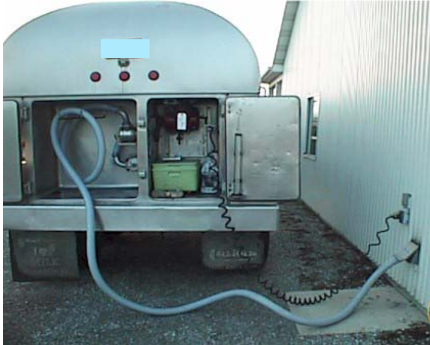
Figure 4 Unloading of a Milk-gathering Truck
