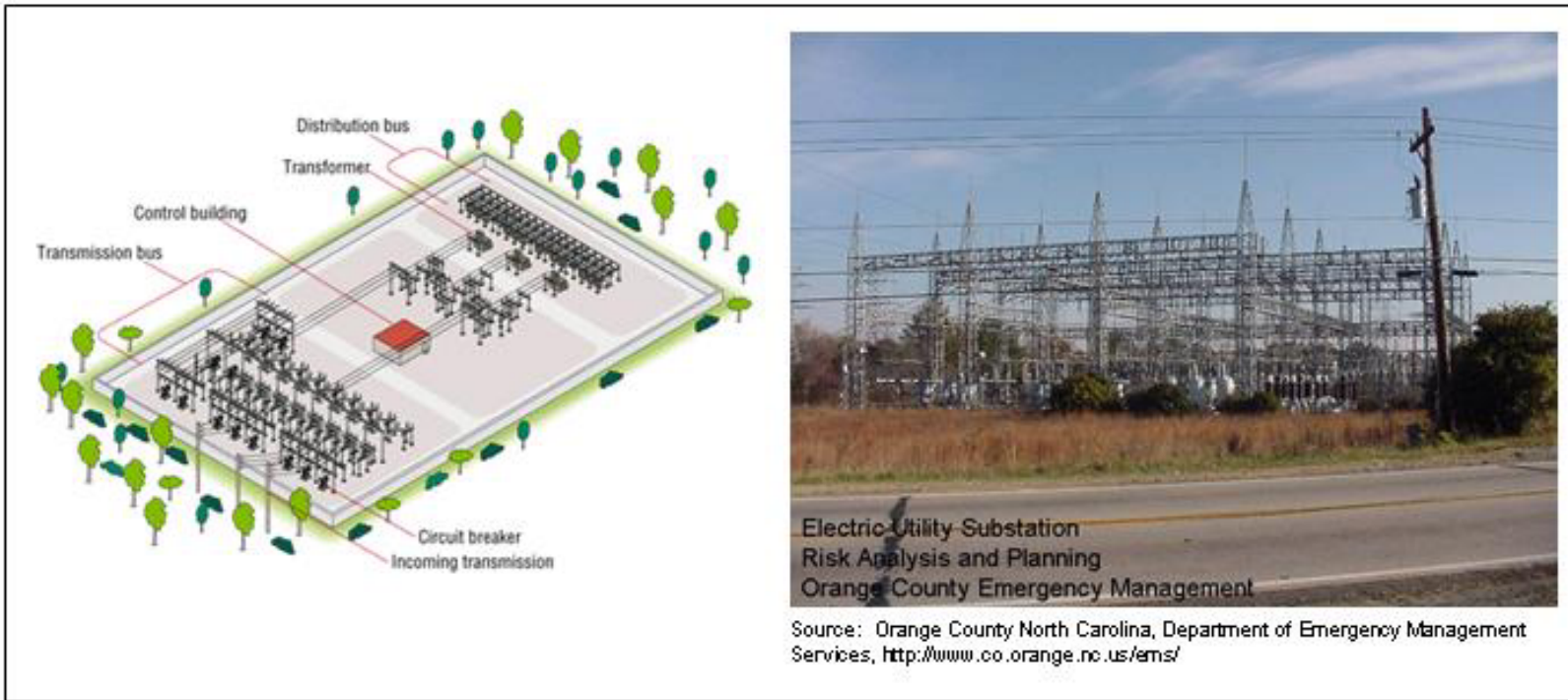
Figure 3 General Layout of an Electric Power Substation
