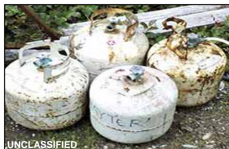
(U) Propane tanks with blue fittings, modified to hold anhydrous ammonia.
