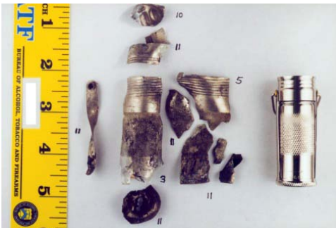
(U) Comparison of matchbox fragments and exemplar
