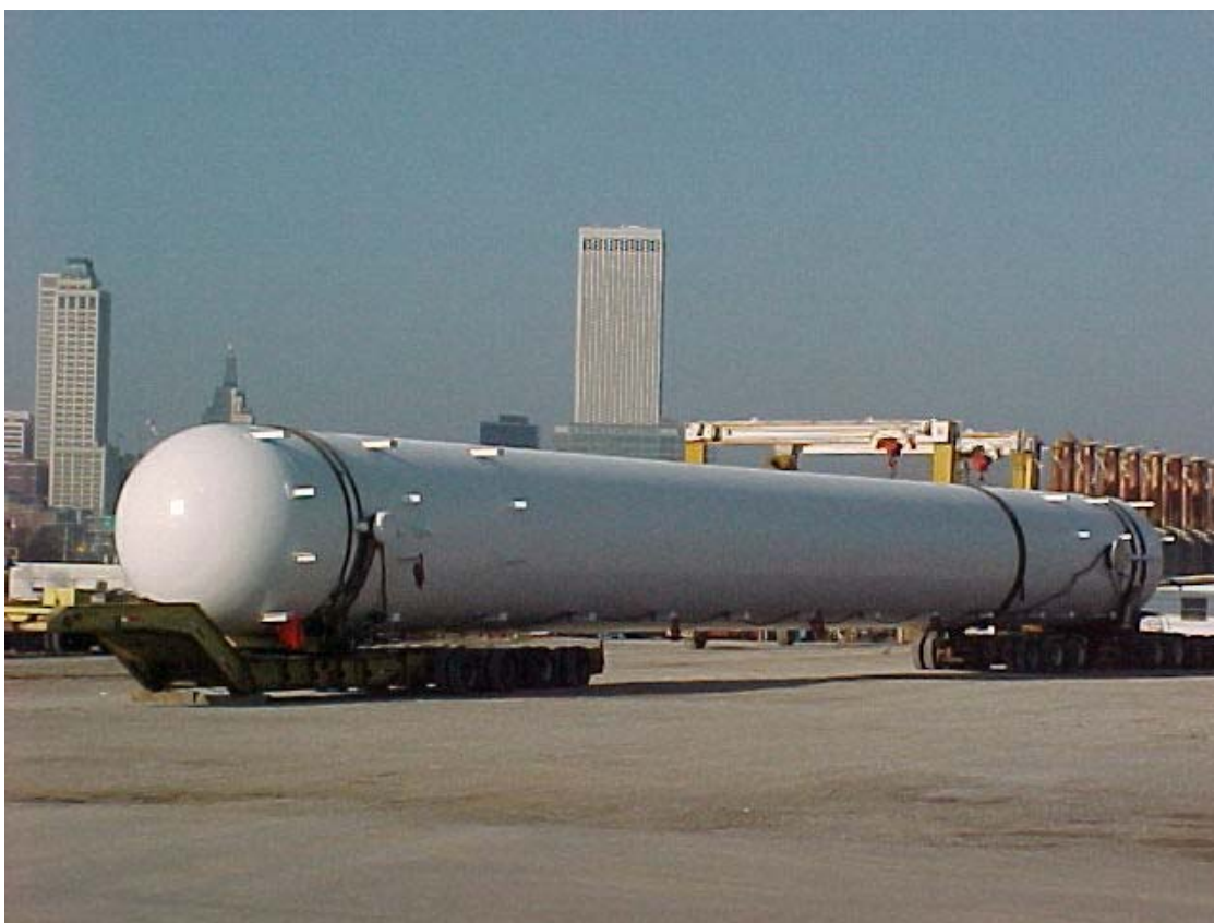
Figure 8-1. Large bulk chlorine storage tank manufactured by Trinity Industries with the flanged man-way located at the far right (bottom) of the tank
