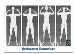
TSA has tested both millimeter wave and backscatter imaging technologies. The new machines are backscatter units. Backscatter technology uses low level X-ray to create a two-sided image. TSA is testing backscatter with an algorithm applied to the entire image to further protect passenger privacy.
