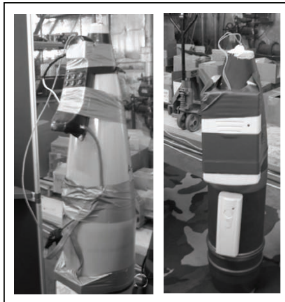
Figure 9-2. Conventional Projectiles Rigged With Explosives and Triggered by Electronic Devices
