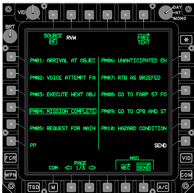
Figure 3-62AE. MSG SEND Page (Source HF)
