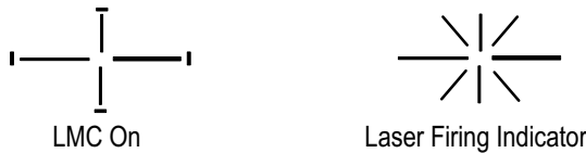
Figure 4-20A. LMC On and Laser Firing Indicators
