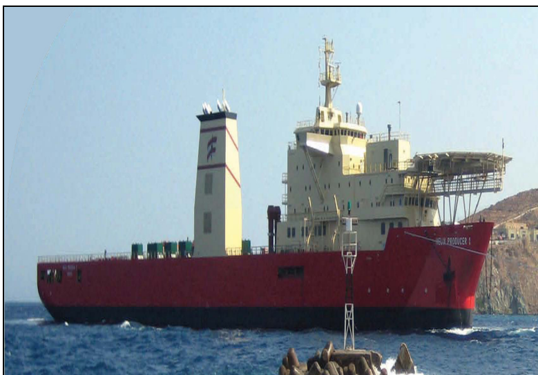
Figure 20. The Helix Producer I , a conventional ship-shape floating production unit. (Photo courtesy of Helix Energy Solutions.)
