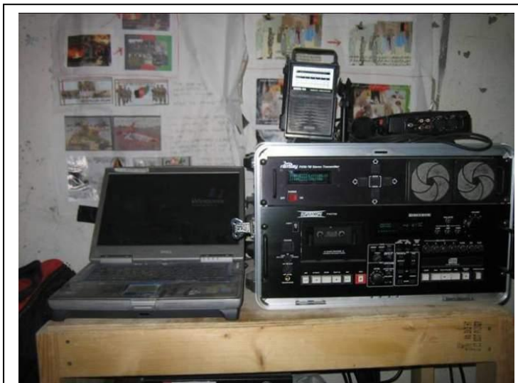
Figure 3: Radio in a Box (RIAB) transmitter with laptop computer, and on top, a hand crank radio.
