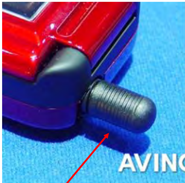
Removal Antenna exposes spray tube
