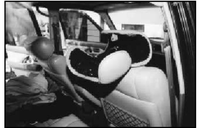
This headrest back flips open like a glove box.
