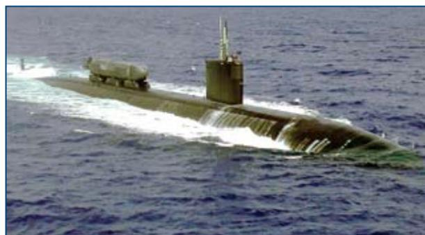
An ASDS rides attached to the top of the much larger Los Angeles Class submarine USS Greenville. The ASDS is connected to the host ship via a watertight hatch. U.S. Navy photo.
