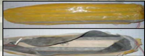
PP -Sealed in Packing Tape & Rubber Inner Tube
