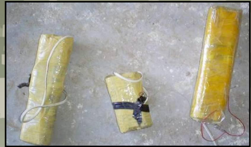
Battery Packs –Sealed in Packing Tape
