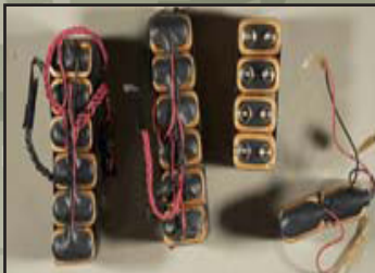
Batteries Taped / Connected Together or Wires Soldered to Terminals
