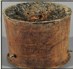
Directionally Focused Fragmentation Charge -DFFC
