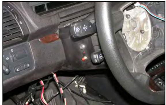
Vehicle Modification: Button to Left of Steering Wheel Caused Emission of Gas under Wheel Wells When Pressed Houston HIDTA Initiative MDS Squad H34/Katy Police Dept
