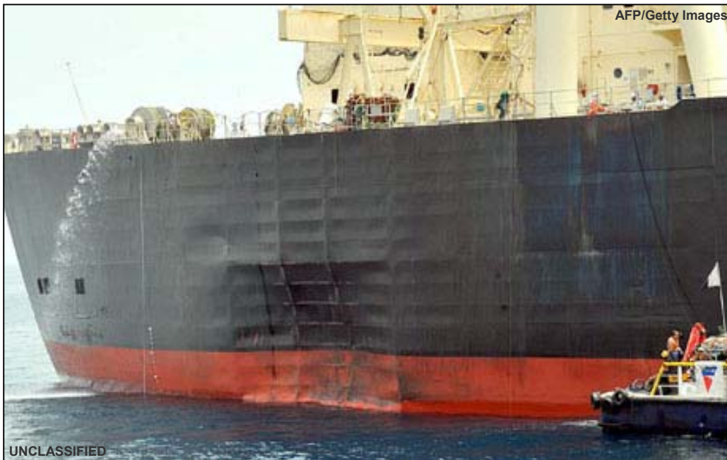
(U//FOUO) Damage from suspected nighttime WBIED attack against M/V M. Star in the Strait of Hormuz.
